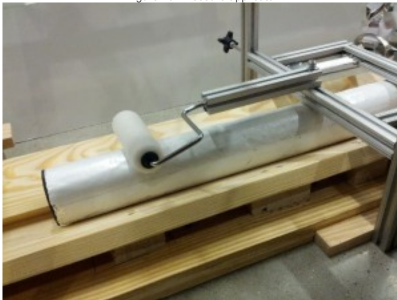
Figure 14: Pressure applicator and foam in place
