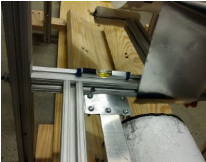
Figure 11: Level indicator to check alignment
